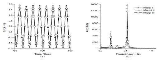
Figure 4: Responses under Regular Waves, WHA=45<sup>0</sup> A) Time History, B) Power Spectrum Density
