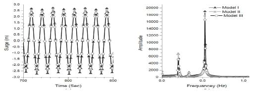
Figure 2: Responses under Regular Waves, WHA=00 A) Time History, B) Power Spectrum Density
