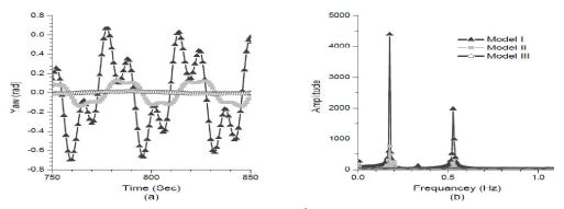
Figure 15: Responses under Regular Waves, WHA=90° A) Time History, B) Power Spectrum Density
