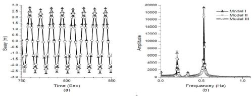
Figure 9: Responses under Regular Waves, WHA=90<sup>0</sup> A) Time History, B) Power Spectrum Density
