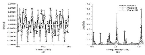
Figure 13: Responses under Regular Waves, WHA=900 A) Time History, B) Power Spectrum Density
