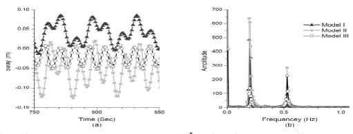
Figure 12: Responses under Regular Waves, WHA=00 A) Time History, B) Power Spectrum Density
