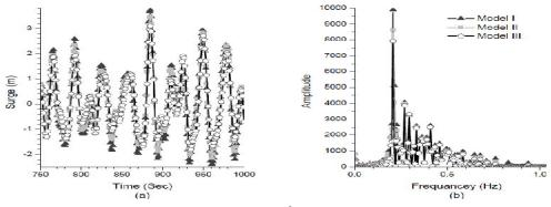
Figure 6: Responses under Random Waves, WHA=0<sup>0</sup> A) Time History, B) Power Spectrum Density
