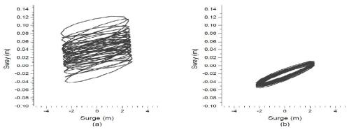
Figure 11: Instability Plane for Surge-Sway (WHA=0°) A) Model I, B) Model III
