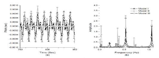
Figure 14: Responses under Regular Waves, WHA=00 A) Time History, B) Power Spectrum Density
