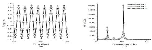
Figure 3: Responses under Regular Waves, WHA=30° A) Time History, B) Power Spectrum Density
