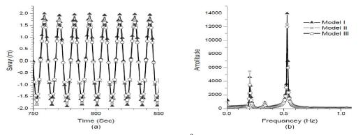
Figure 8: Responses under Regular Waves, WHA=45<sup>0</sup> A) Time History, B) Power Spectrum Density
