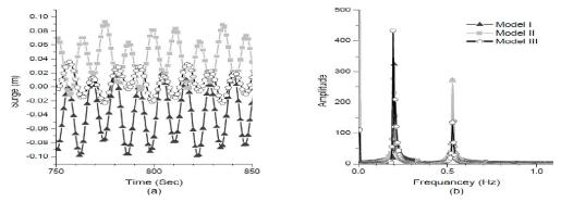
Figure 5: Responses under Regular Waves, WHA=90° A) Time History, B) Power Spectrum Density
